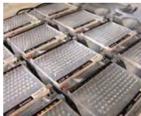
Figure 13 – Over twenty E-Gel® 48 or E-Gel® 96 gels can be run at once
