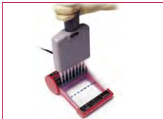
Figure 4 – Sample loading and electrophoresis results using double comb E-Gels
