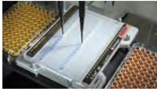
Figure 8 – Loading an E-Gel® 48 gel using a liquid handling robot
