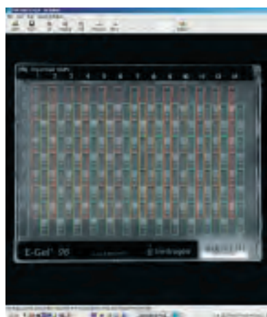
figure 6 - the E-Gel® 96 Editor software reconfigures the E-Gel® 96 gel's staggered-well format
