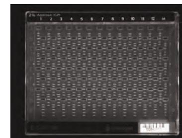
Figure 1B. Electrophoresis result using the Tango Automated Liquid Handling System and the Invitrogen E-Gel 96 system. Sample: E-Gel 96 Low Range DNA Marker (90ng).
