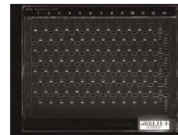
Figure 1A. Electrophoresis result using the Tango Automated Liquid Handling System and the Invitrogen E-Gel 96 system. Sample: 1m (50ng) of b-actin PCR product (length: 838bp), DNA marker: E-Gel 96 Low Range DNA Marker.
