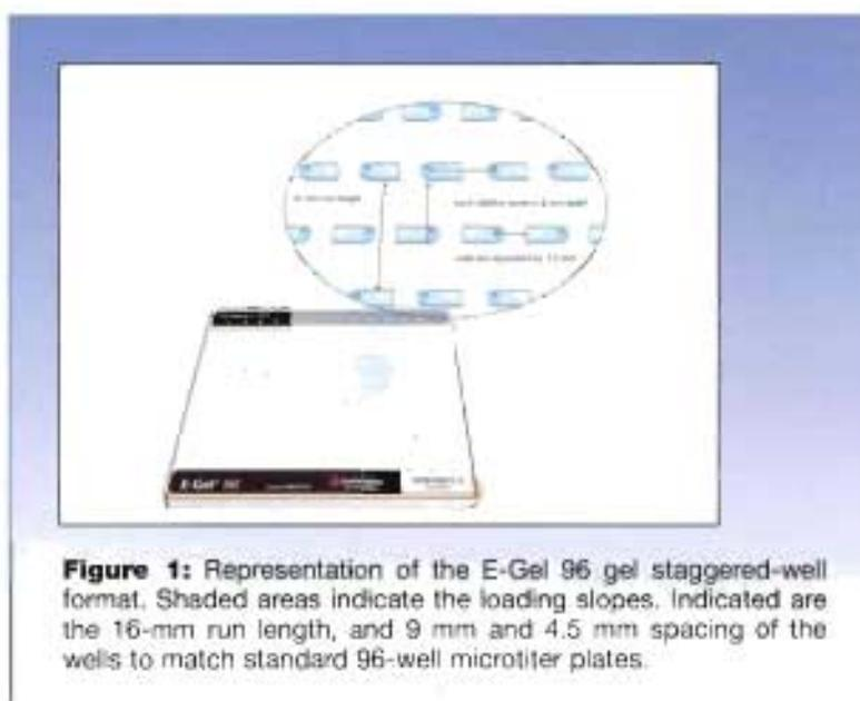
**Figure 1:** Representation of the E-Gel 96 gel staggered-well format. Shaded areas indicate the loading slopes. Indicated are the 16-mm run length, and 9 mm and 4.5 mm spacing of the wells to match standard 96-well microtiter plates.
