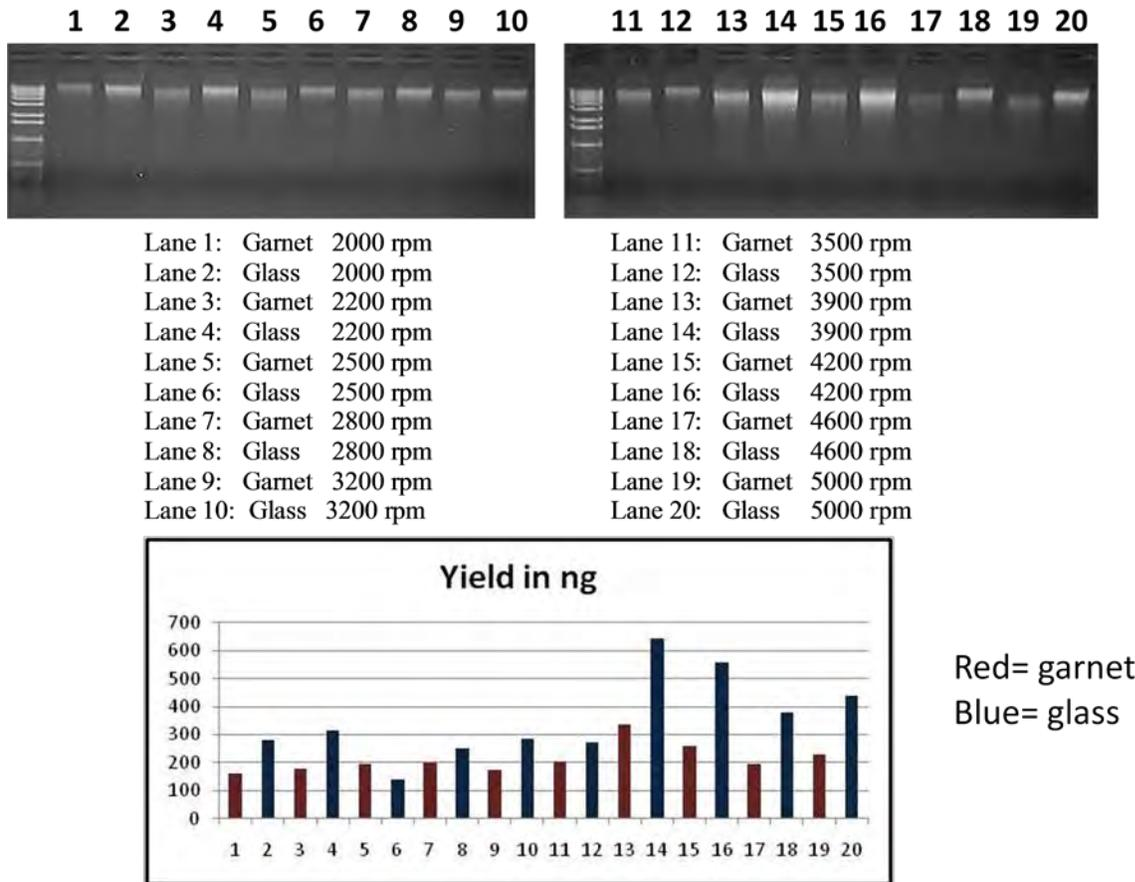
**Figure 1. DNA isolation from clay soil (soil 1) with increasing speed for 45 seconds.** DNA yields remain consistent with either glass or garnet bead tubes until speeds reach 3,900-4,200 RPM where maximum DNA recovery is achieved using glass bead tubes. DNA yields decline when the bead beating speed exceeds 4,200 RPM, indicating that too much force can be detrimental to DNA recovery.
