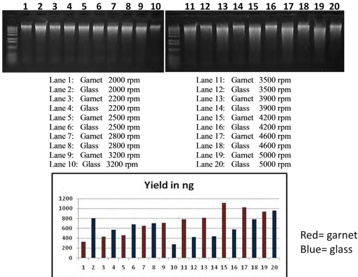
**Figure 2. DNA from silty clay soil was extracted using the PowerLyzer™ 24 Homogenizer with increasing speed for 45 seconds.** DNA yields demonstrate that soil 2 performed better with less vigorous bead beating and that the garnet bead tubes performed equally as well as the glass bead tubes. Optimal DNA yields were achieved at lower speeds using the glass bead tubes while the garnet bead tubes required higher speeds for maximum DNA yields.
